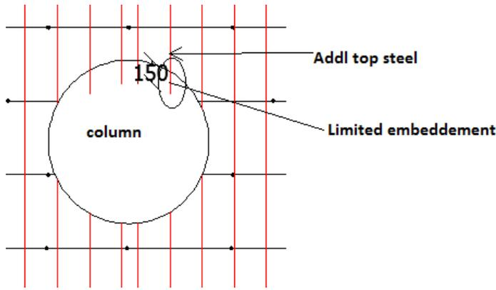
**Fig 7: Limited embedment of top and bottom steel at columns**
