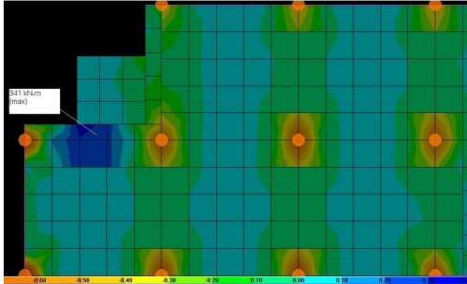
**Fig 5 : Moment Contours in Y direction**
