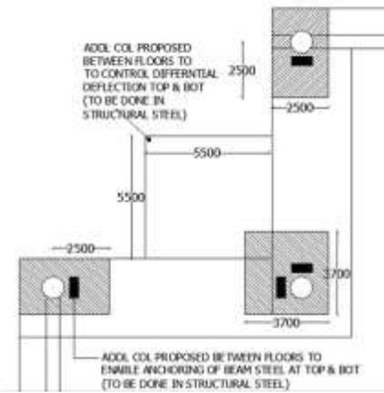
**Fig 8: Proposed additional columns with heads**
