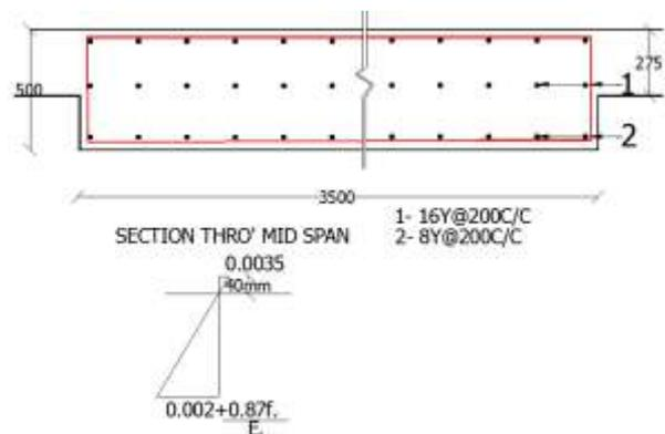
Fig 2: Section through Mid span showing provided steel & corresponding strain diagram
