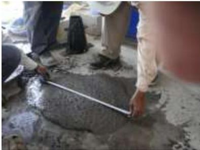
Fig. 13. : Micro concrete spread test
